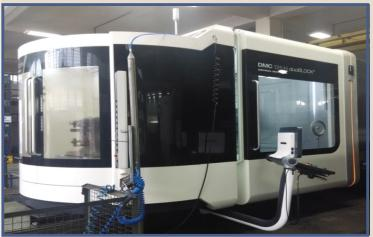
With a table size (L X W in mm) of 800 x 800, large traverse paths could be achieved and a high pallet load up to 2,000 kg are possible with the new space-saving pallet-exchange design & rear chip disposal.
