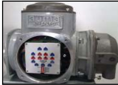
Fig. G: 1.XMP Module within EPAC enclosure
