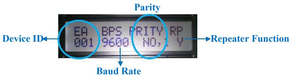
If the above displayed settings are not matching with the intended options for Modbus communication, then for changing the Modbus parameters, use the below flowchart.
