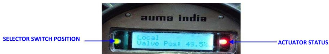
Fig. C: LEDES ON THE FRONT PANEL
