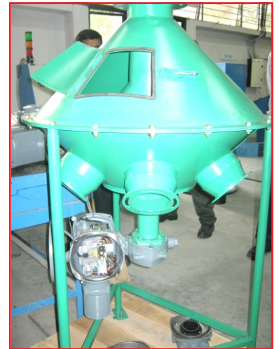
AUMA India actuator and gearbox in use with 5-port valve
