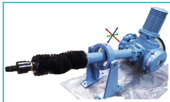
New Trunion Mounting Arrangement with horizontal and vertical movement
