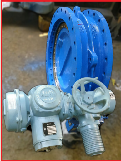
AUMA India actuator installed on butterfly valve of R&D Multiples at their facility
