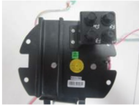
POWER MODULE ASSY-1.XMP-1TFR. EPAC [TFR. ASSY + FUSE ASSY]
