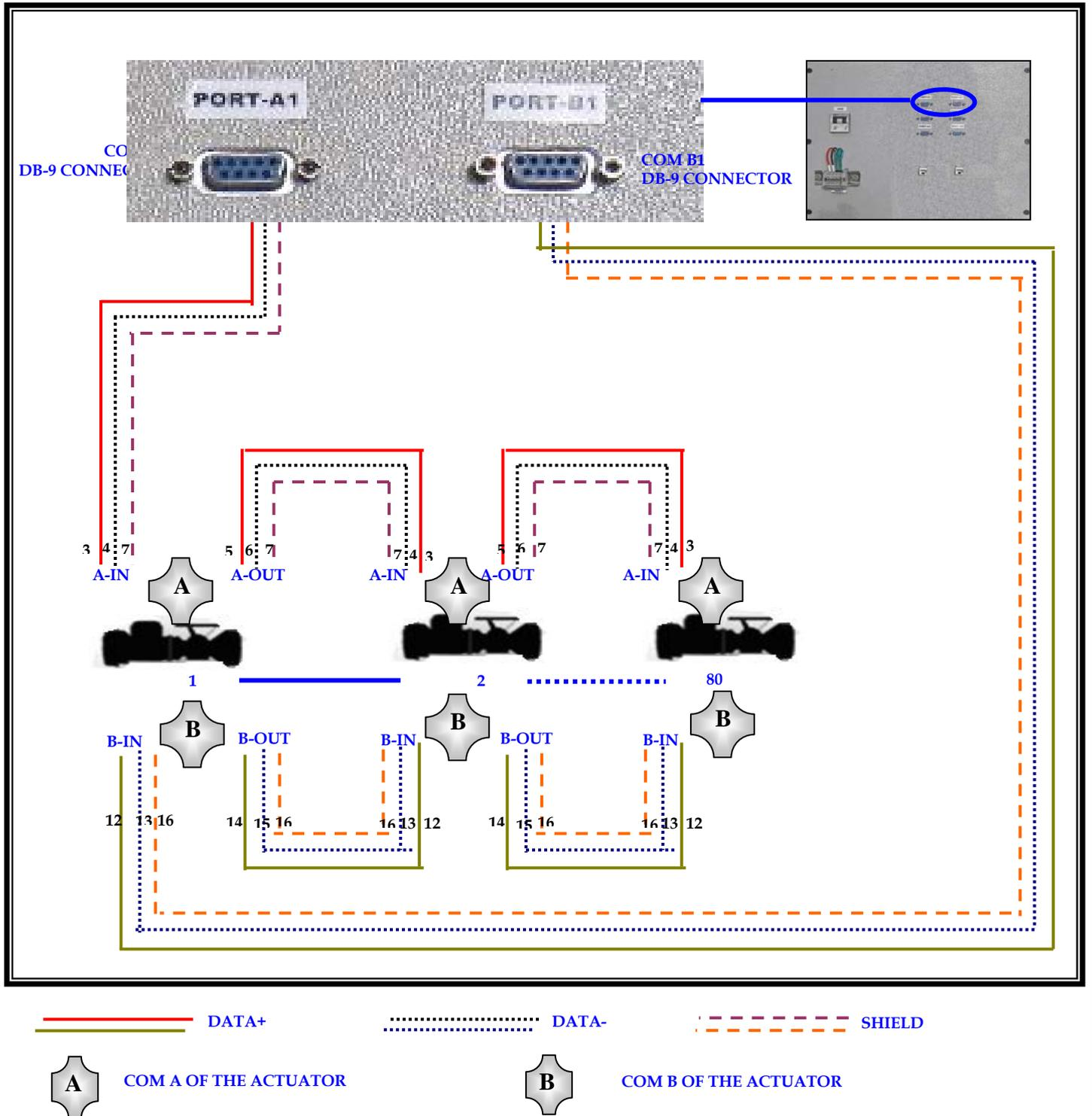
FIGURE 9: AIMS REDUNDANT LOOP TOPOLOGY
