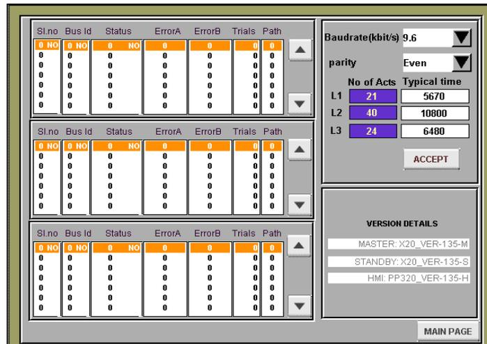
This is the information window, which shows the version details and the Communication settings of the actuator connected in each loop (do not edit these settings)
