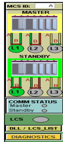
The red color on the Loop (A or B) as shown below, indicates the failure of the particular channel (In the below figure, it indicates the failure in channel B of Loop2 & Line break at Loop1)
