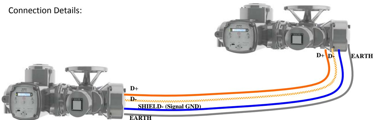
**FIGURE 5: INTERCONNECTION BETWEEN FIELD ACTUATORS**
