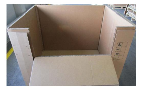
The goods inside the carton should be secured against damage with filling materials according to the delivery conditions. The carton is closed with a slip lid and 2-fold banded. In case of corrosion-sensitive components, the carton must be lined with a VCI bag.
