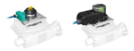
The inductive sensor switch records and signals the valve end position. It is used in combination with GS .3 part-turn gearboxes and is particularly appropriate for position monitoring of manually operated valves.
