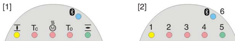
Figure 37: Arrangement and signification of indication lights
